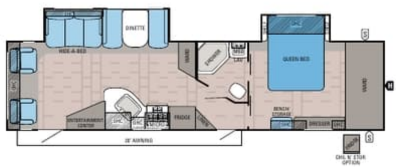
WHITE HAWK | 33RLBS OPTIONS: A, D Ext. Lgth: 37' 11" Ext. Ht: 136" Unloaded Wt (lbs.): 7,235 Sleeps: 4-6
